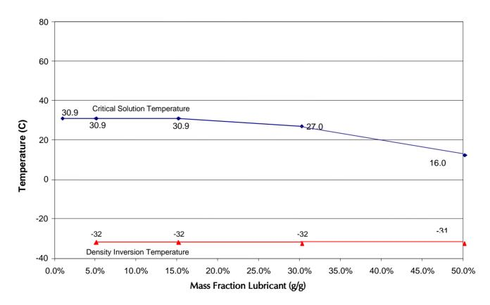
An upper critical solution temperature, consistent over a wide range of lubricant concentrations, is observed for the **GEOlube**<sup>®</sup> **RFL** grades. A low temperature critical solution temperature does not occur, although a density inversion in the liquid phases is observed over the full lubricant concentration range tested.
