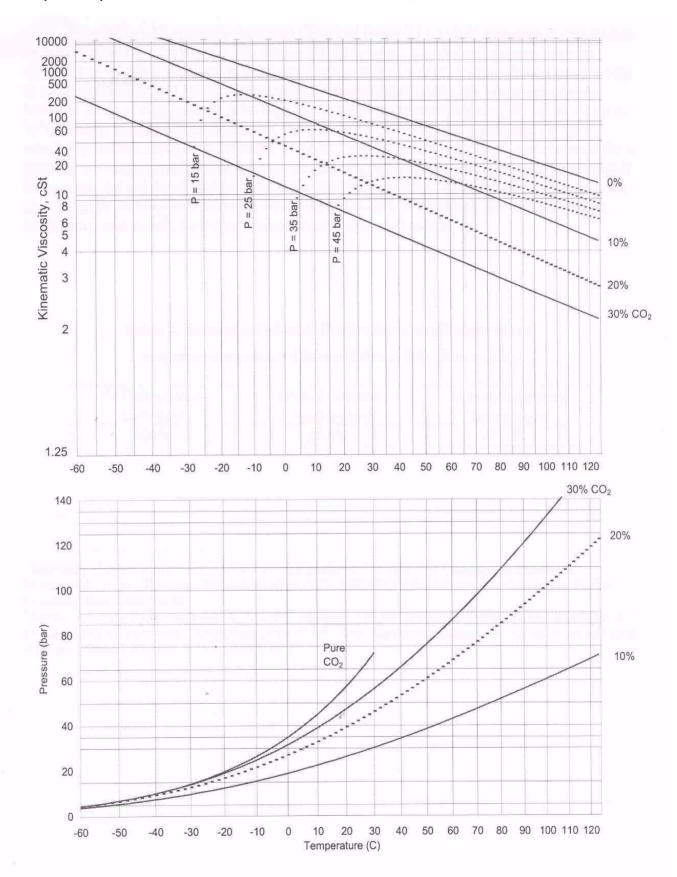
Viscosity and Vapour Pressure Data for GEOlube® RFL 100X / CO2
