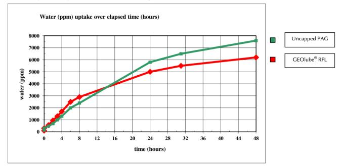
Water Absorption Properties of GEOlube® RFL grades
