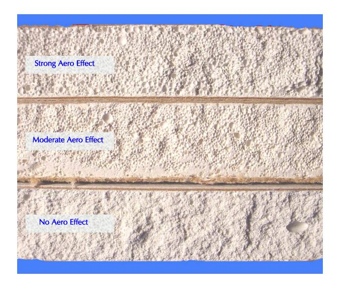
**Aero<sup>TM</sup> Technology** gives gypsum board manufacturers unparalleled flexibility. The degree of effect can be controlled depending on product and operational choices, allowing the balance between strength, weight and kiln energy requirements to be optimized •
