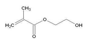
Bisomer<sup>®</sup> CL HEMA (Hydroxyethyl Methacrylate) is widely used in the preparation of long-term wear or disposable contact lenses.
